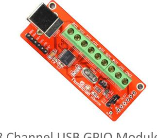
8 Channel USB GPIO Module
